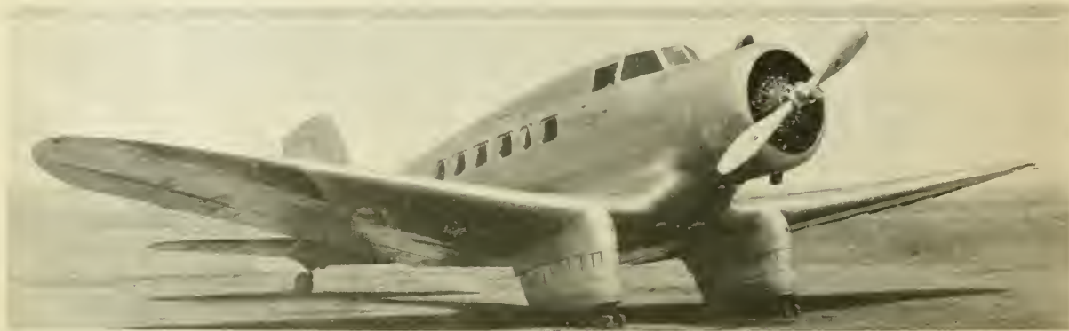
715 h.p. Wright Cyclone-powered Executive model recently introduced by the Northrop Company
